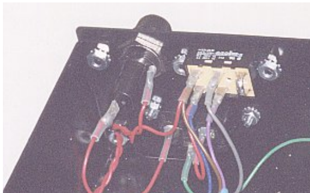
Figure 1 Power entry with voltage selector switch.
