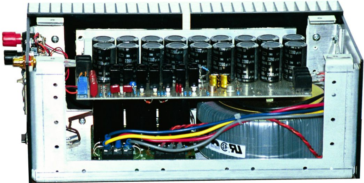
Figure 3: Inside view. Note the placement of the MB301 power amplifier board (mounted on heatsink on the side of the unit) and the PS11 power supply board; (mounted onto the bottom of the chassis) . The toroidal power transformer is mounted near the front of the unit on the baseplate.
